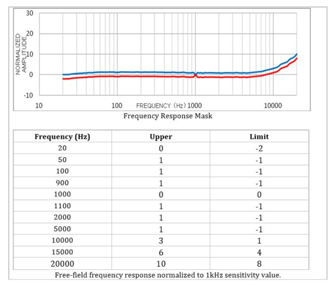
Frequency Response Mask (100% Pass/Fail Test for Microphones)
