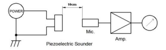
MIC: ND10 Sound Meter or equivalent DC Power Supply: QJ6003S or equivalent
