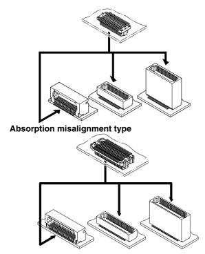
This JMC connector is 0.5mm pitch SMT type board to board connector with selection of boss existence. Comparing with conventional JMC connector, more small and space saving are realized. Various types are available such as top/side entry type connectors including the development of the stacking height variation for plug and the absorption misalignment type for receptacle.
